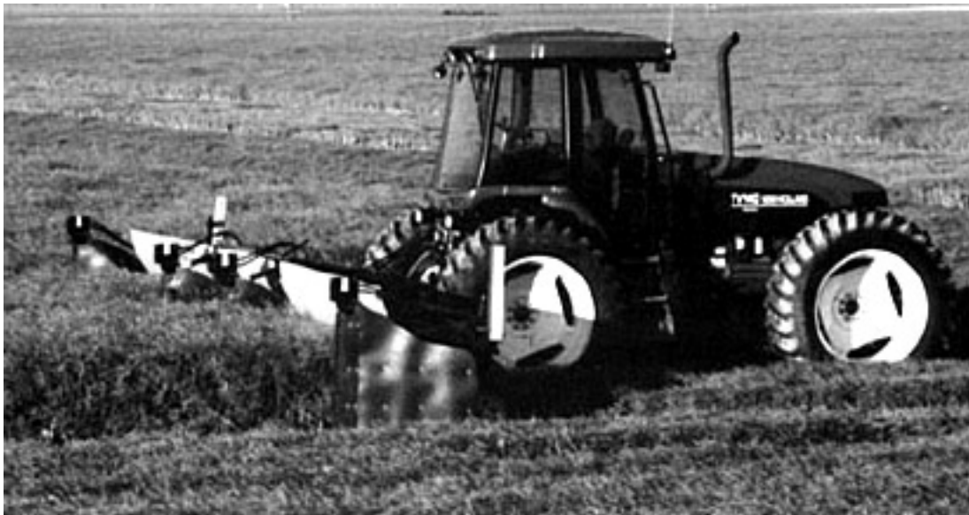
Figure 1. The Yield Shield from AgShield of Canada is used to bend canola stalks while green, which the company claims encourages a more uniform ripening of seed without cutting the plant. Note: The steering mechanism on the tractor swivels, so it is actually driven backwards!
